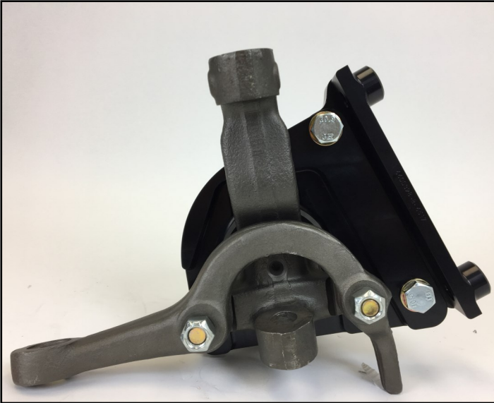
12. Picture of the radial bracket installed to the base bracket. (Inboard view)
