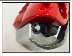
Install the pin from the backside of the caliper into the groove on the anchor. (Where the 'S' clips are) The pin should go all the way through to the front of the caliper. Install the 'E' clip onto the groove on the end of the pin to secure the anchor to the pads. Repeat this process for the other caliper. Now you are ready to install the caliper onto the rotor.
