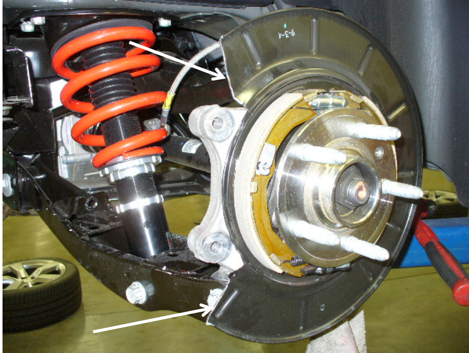
Trim shield in areas indicated by arrows. This shield has been trimmed.
