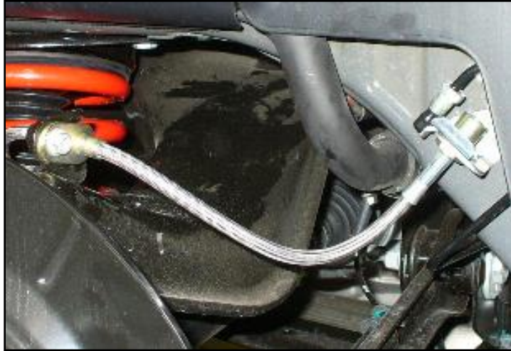
Figure 4: Proper Hose Installation
