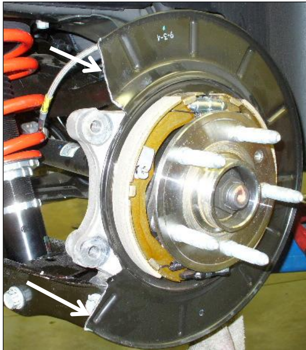
Figure 1: Modified Debris Shield
